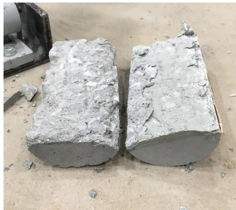
Figure 5.22 Cylinder 2 split cylinder failure (Ruble)
