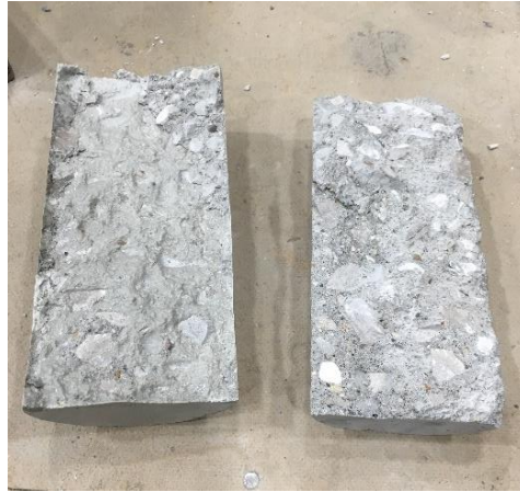
Figure 5.21 Cylinder 1 split cylinder failure (Ruble)
