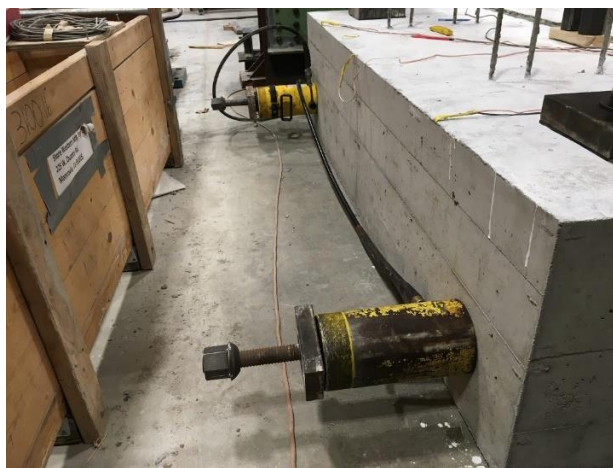
Figure 5.25 Actuators used to mimic thermal loading (Ruble)
