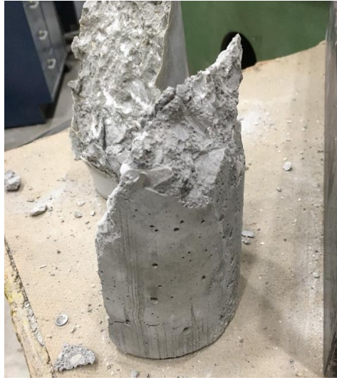
Figure 5.17 Cylinder 2 slant shear failure (Ruble)
