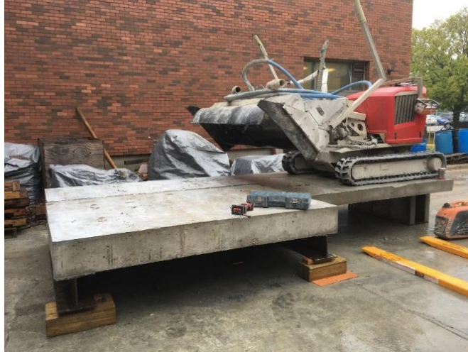
Figure 5.9 Aquajet aqua cutter 710H (Ruble)
