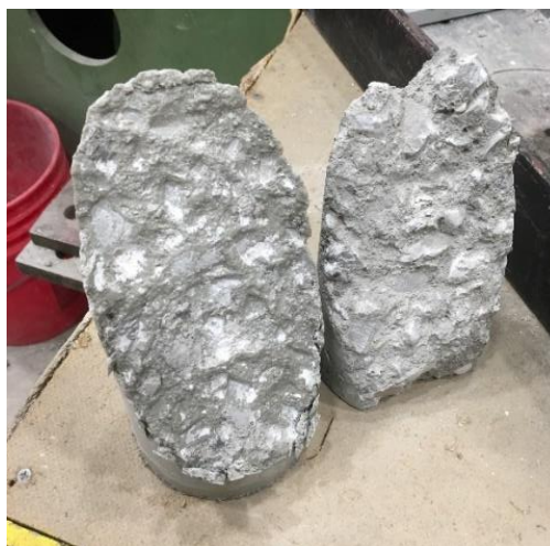
Figure 5.16 Cylinder 1 slant shear failure (Ruble)
