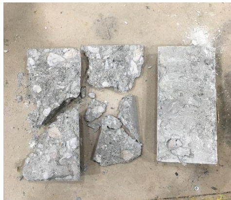
Figure 5.23 Cylinder 3 split cylinder failure (Ruble)
