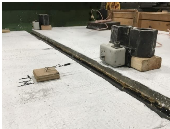
Figure 5.10 String potentiometer (Ruble)
