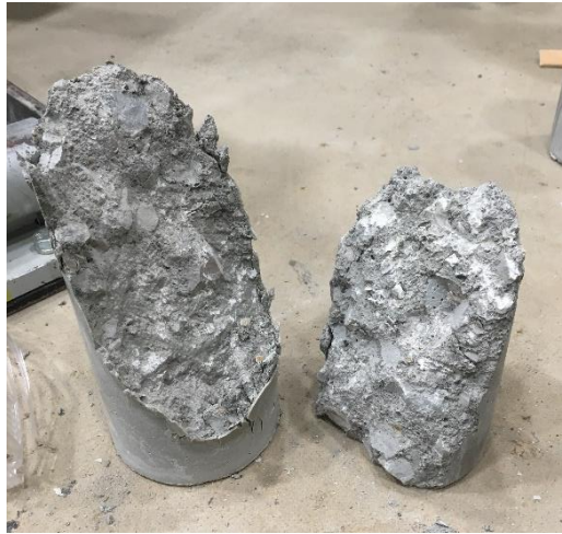
Figure 5.18 Cylinder 3 slant shear failure (Ruble)
